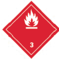
Figure 2 Pictogram for Flammable Liquids used in the UN Model Regulations (Symbols: fire: black or white; background: red; the figure of 3 is at the lower part; the minimum size: 100mm x100mm)
